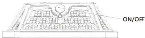
Notes: If there's sunlight or other lights on the solar panel, the lamp will not be on even if the ON/OFF switch has been turned on. During testing, other object should be used to cover the solar panel, then the lamp will be on after turning on the ON/OFF switch.
